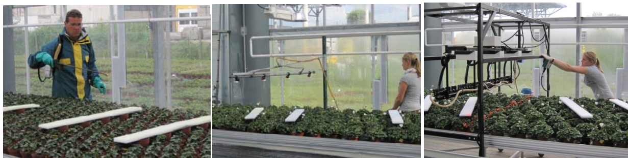
Fig. 2. Spray techniques used in cyclamen pot plant spraying; hand held lance (left), spray boom (center) and CAS-sprayer with sensors to detect individual plants (right).
