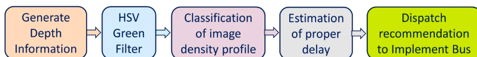
Fig. 3. The information flow from the detection of the canopy to the recommendation of the spraying rate.
