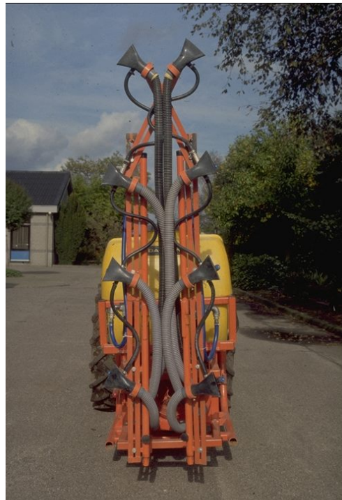
Figuur b. De experimentele spuit. Figure b. The experimental cross-flow fan sprayer.
