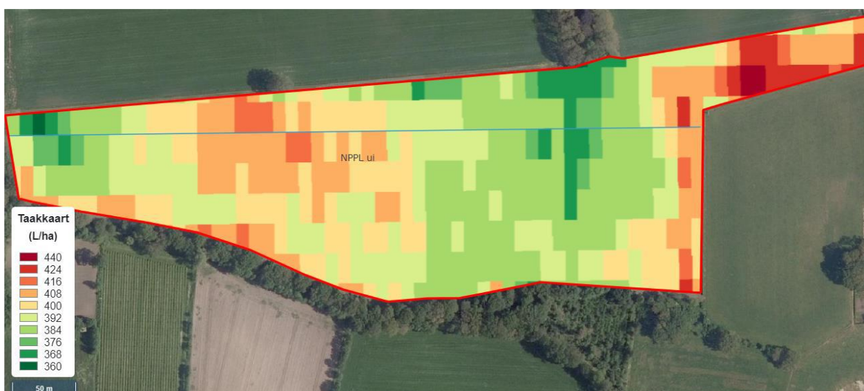
Figure 4 Task map of the treated field showing the spraying volume (L/ha; Note 400 L/h spraying volume equals 1.4 L product/ha) adjusted to a 24 m working width boom sprayer. Figure taken from van Boheemen et al. (2022).
