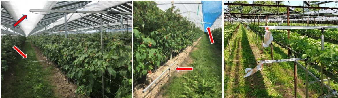
Fig. 2. Left: PARbars above and below raspberry in agrivoltaics. Middle: raspberry control under plastic. The lower PARbar is in temporal position parallel to the row for traffic to pass. Right: strawberry.
