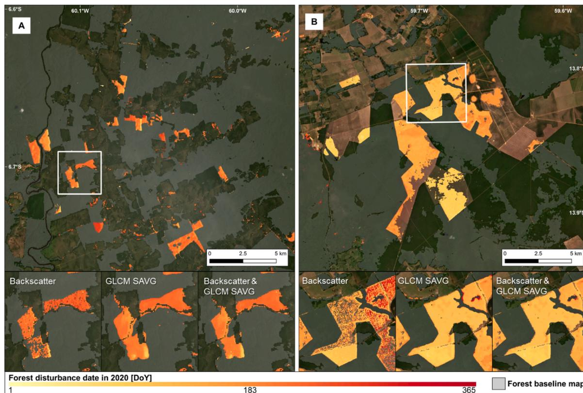
Fig. 6. Forest disturbance dates [DoY] for combinations of backscatter and GLCM SAVG (kernel size 7) data for Site 1 (A) and Site 2 (B). Detailed maps are given for disturbances mapped based on backscatter (bottom left), GLCM SAVG (bottom middle) and a combination of both (bottom right). Combination results for all sites can be visualized via <https://johannesballing.users.earthengine.app/view/forest-disturbance-texture>.
