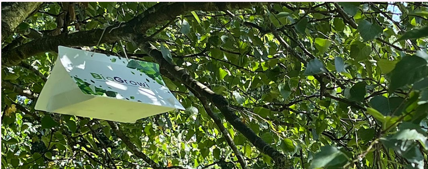
A fungus trap catches airborne spores on an adhesive strip • Photo Bo Briggeman
