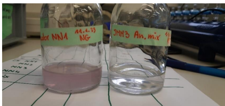
Figure 6 Medium with resazurin solution in oxygen (on the left) and anoxic conditions (on the right).
