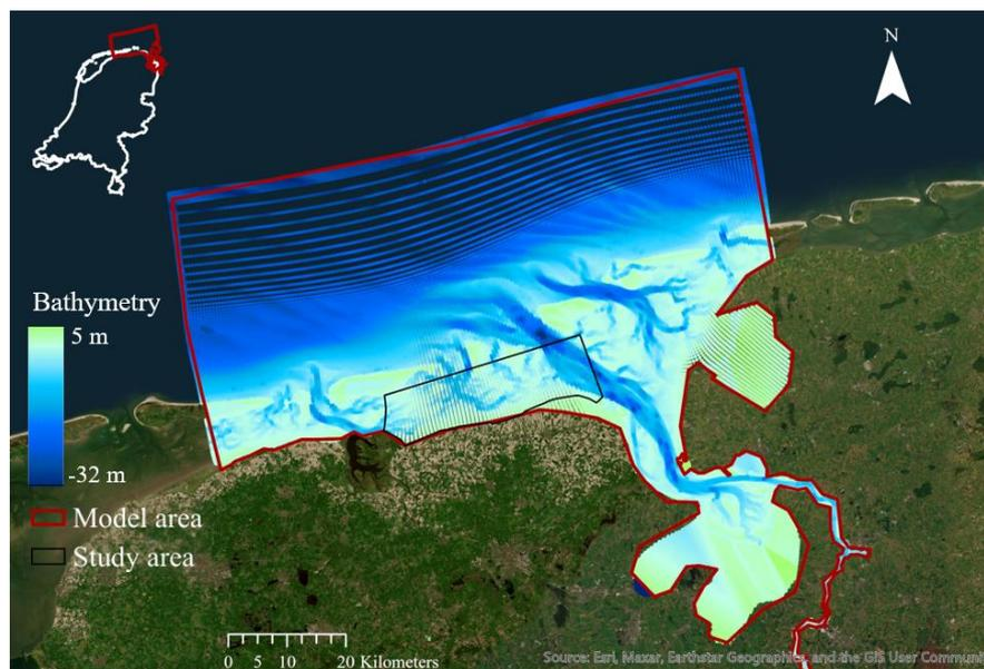
Figure 3. The modelled Ems-Dollard estuary (red) and the study area (black) with the initial bathymetry (m compared to NAP).
