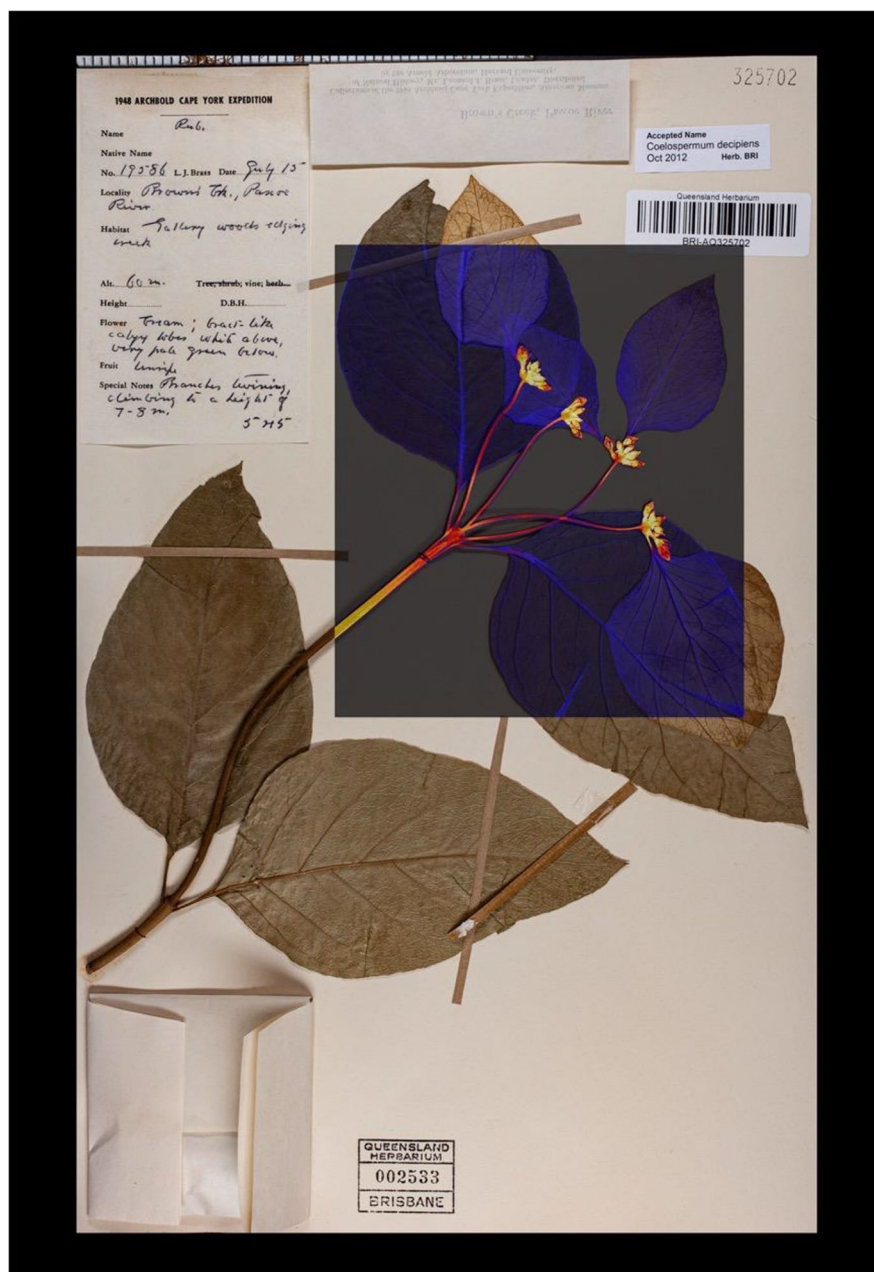
Fig. 2 Laboratory \mu -X-ray fluorescence elemental map (1300 \times 1129 pixels) overlaid over a photograph of an herbarium specimen ( Coelospermum decipiens ) that was found to hyperaccumulate Se. The brighter shades in the elemental map denote higher Se concentrations
