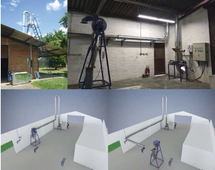
Fig. 4.4 Flash-dryer prototype installed at CIAT
