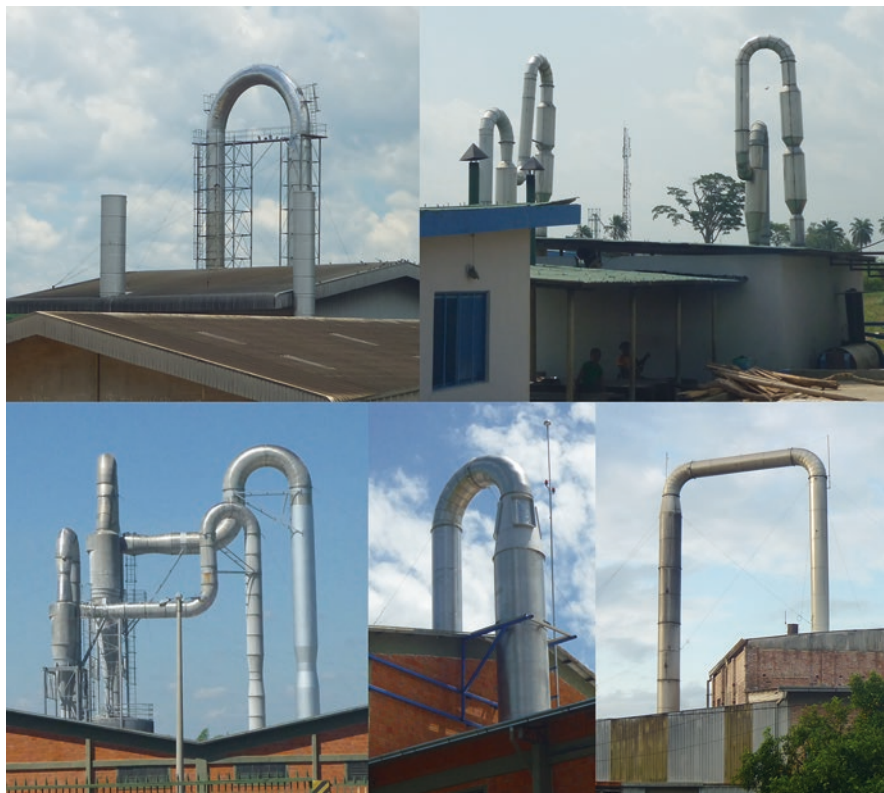
Fig. 4.2 Diversity of flash-dryer designs in Thailand, Nigeria, Paraguay (dryer model from Brazil), Paraguay (dryer model from Sweden), and Argentina
