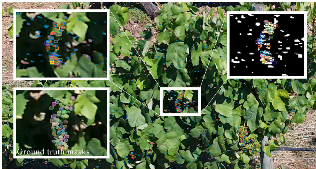
Fig. 7. YOLACT detection of berries. On the top left it is zoomed in with the predicted grape masks, and in the bottom left with ground truth masks.
