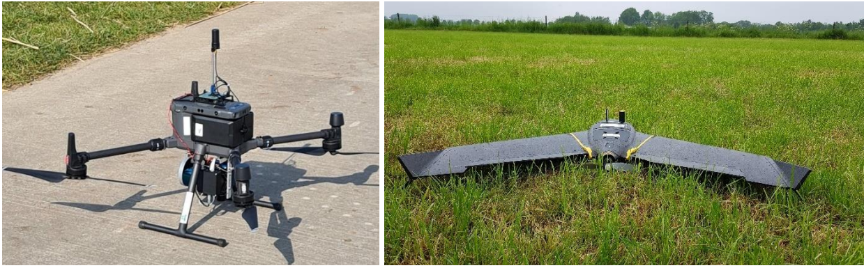
Figure 2.2 Multicopter with hyperspectral and LiDAR camera, Nano Hyperspec (Left) and a EBEE fixed wing drone with multispectral camera (Right).
