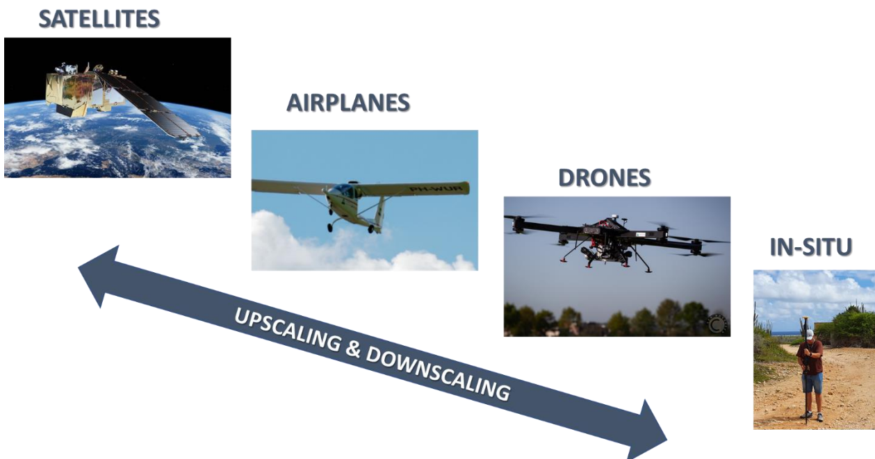
Figure 2.1 Multi-scale sensing approach with different remote sensing platforms: spaceborne, airborne and ground-based.
