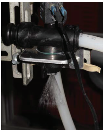
Fig. 1. PWM-nozzle used in the experiments.
