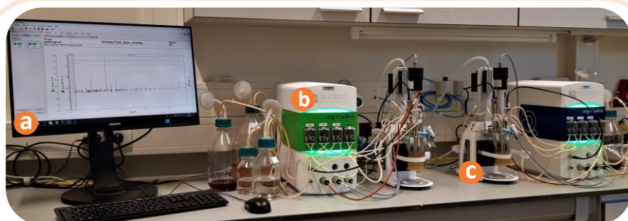
Figure 1. Continuous single-stage fermentation culture system (Applikon®). a. Process control software (semi-automated workflow & real time monitoring) b. Advanced process controller (simulation of the broiler's caecal physiological conditions) c. Small-scale bioreactor (250 ml).
