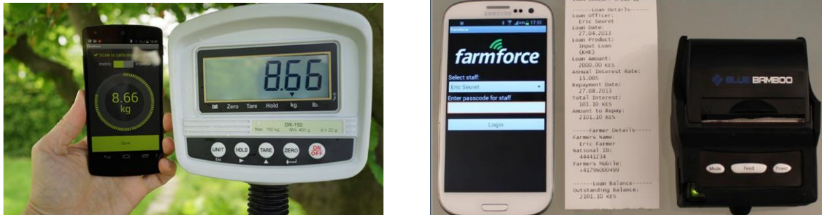
Figure 2: The wireless scale (left) and Bluetooth printer (right) which are key in managing accurate traceability. (Courtesy: Farmforce)
