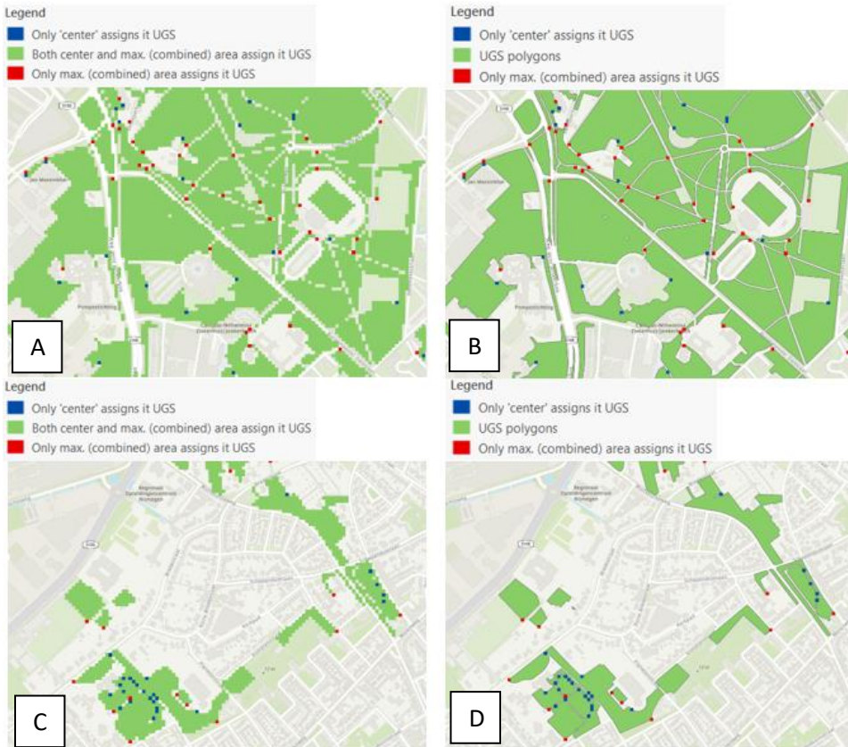
Figure 26 Polygon to raster transformation of UGS with Cell center method and Maximum (combined) area compared for two different sites. The left images show the raster data (A) and (C), and the right shows the vector data (B) and (D).
