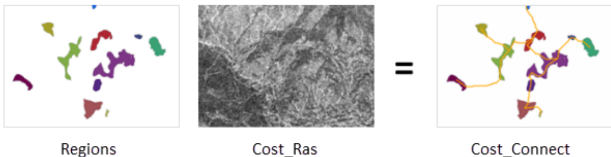
Figure 9 How the Cost Connectivity tool works: input regions and a cost raster result in an output of a least-cost network over the regions (ESRI, n.d.-a).
