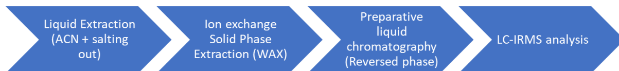
Figure 3.3 Schematic overview of the developed clean-up for 2-thiouracil in bovine urine samples.
