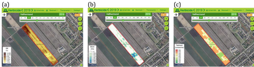
Fig. 5 Three steps in the soil herbicide apps. (a) Upload of soil organic matter map, (b) herbicide prescription map, and (c) machine-ready task map
