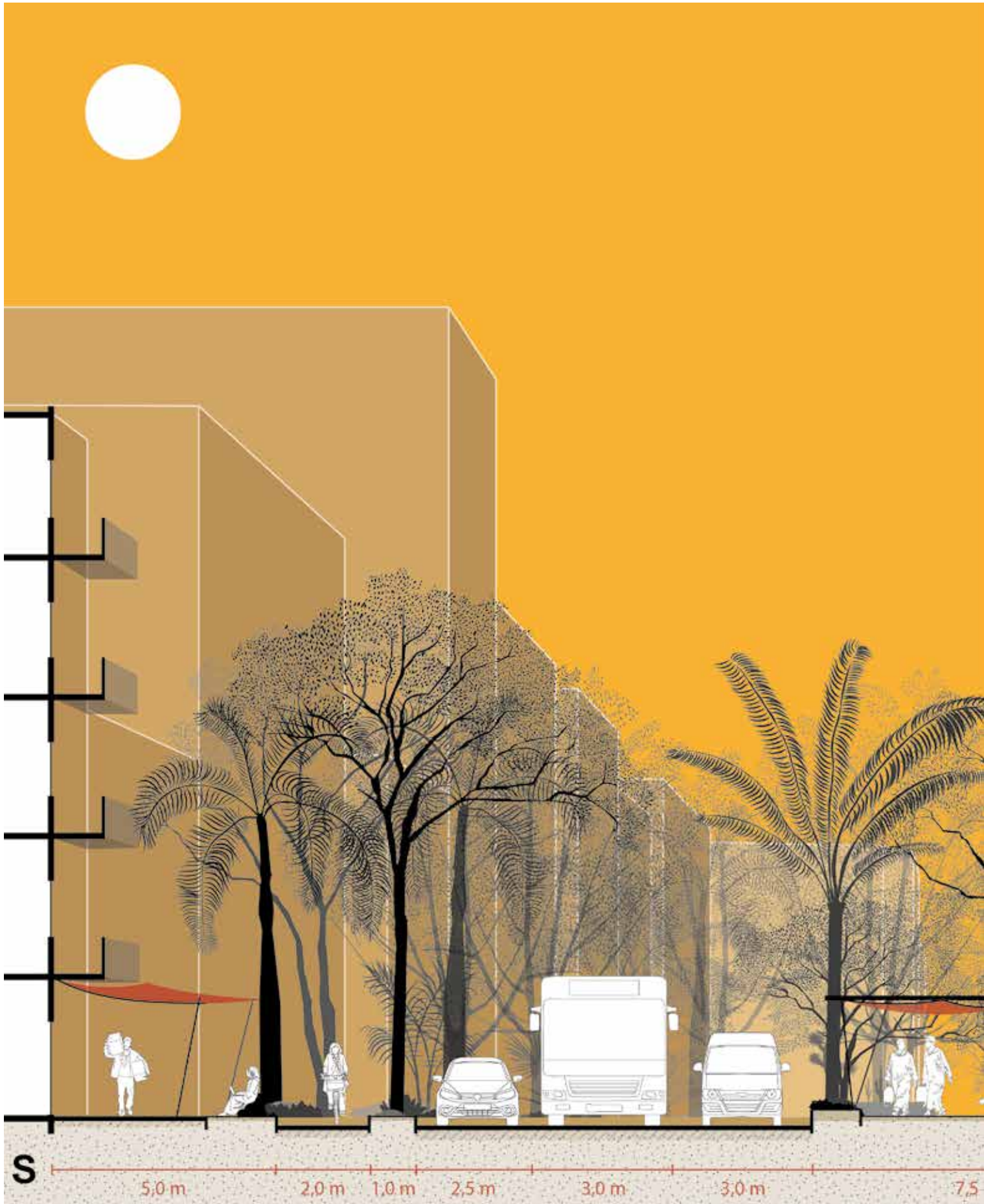
B Fig. 62 Section of detailed design 2, illustrating the several shading methods applied to shade pedestrian areas as effectively as possible.
