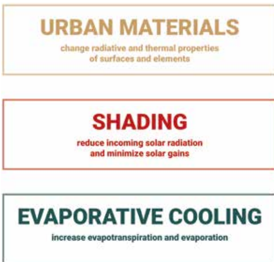
Fig. 7 Overview of the three cooling strategies, the different color assigned to each strategy indicates to which cooling strategy each design intervention contributes.
