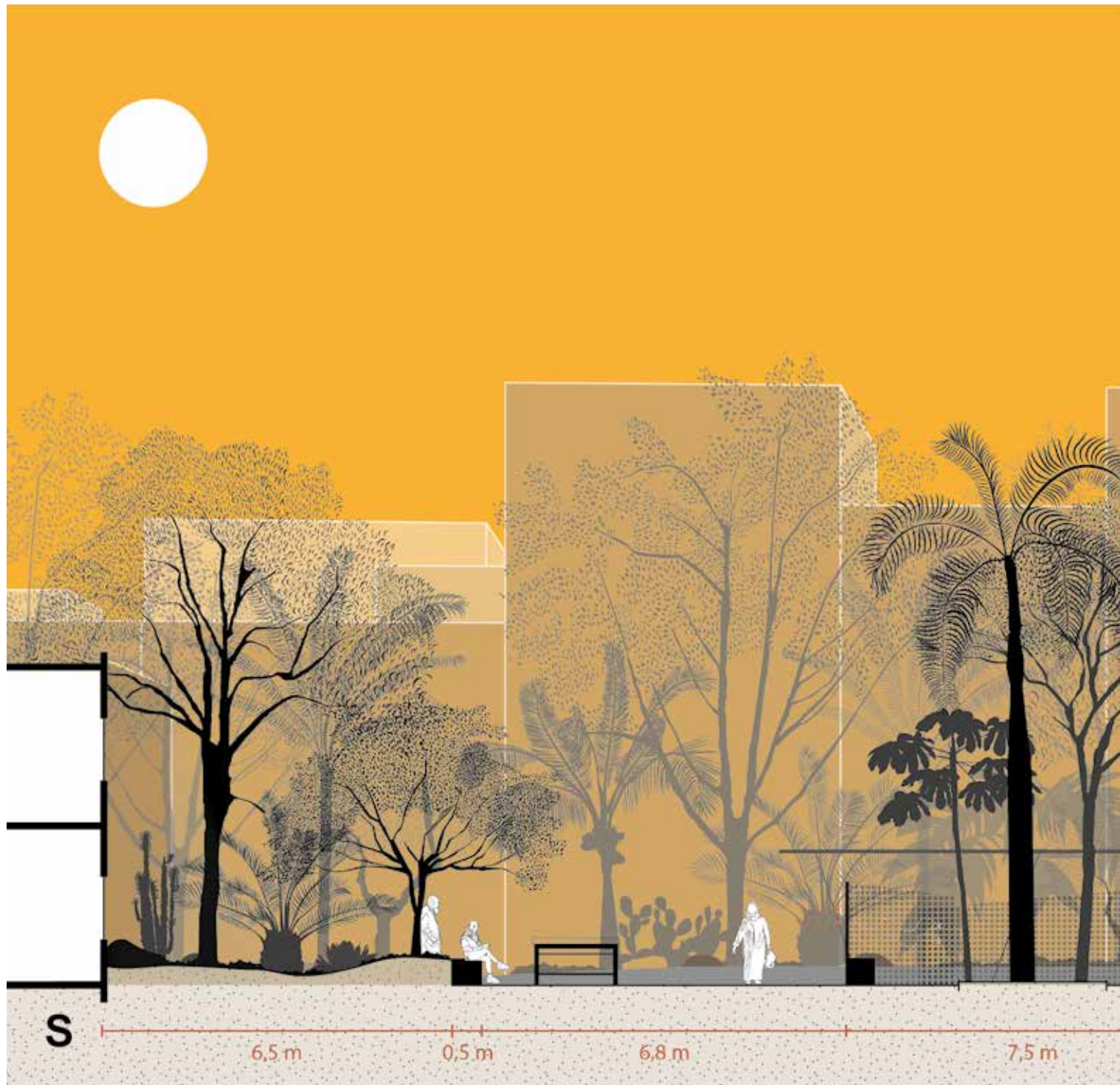
A Fig. 60 Section of detailed design 1, illustrating the planting beds with the varying vegetation, ping pong table, evaporative wall, and free-standing louvres with canvas canopies.
