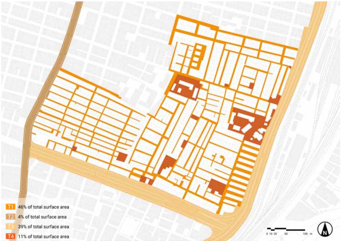
Fig. 35 Spatial overview of the representative street typologies T1-T4 and their distribution at the Shubra district.
