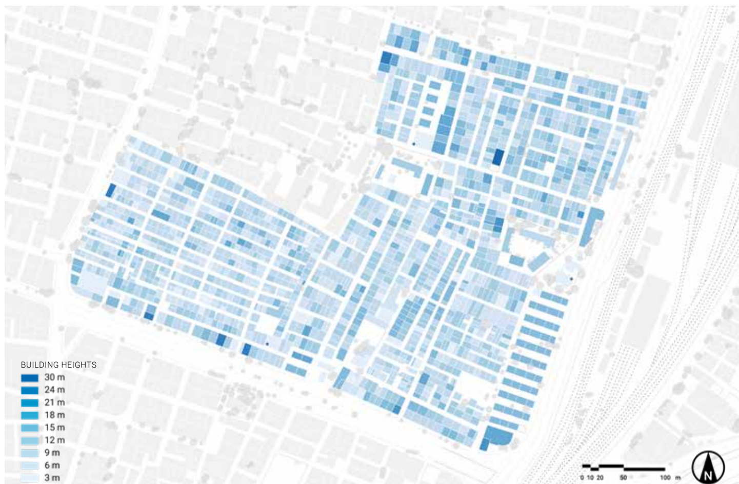
Fig. 43 Map of building heights in the study area (ranging from 3 to 30 meters), showing an irregular pattern with a high surface roughness (based on a GIS analysis; data received from Ain Shams University).
