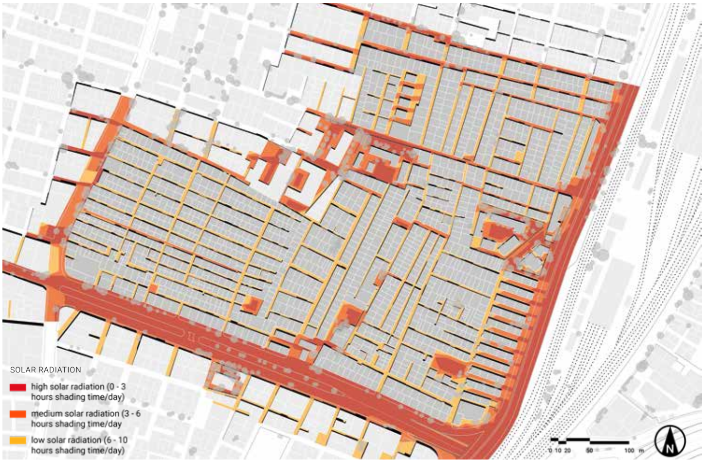
Fig. 47 Map of solar radiation that the study area receives, expressed in amount of shading hours per day. Based on the Shadow Analysis plugin in Sketchup 2021.
