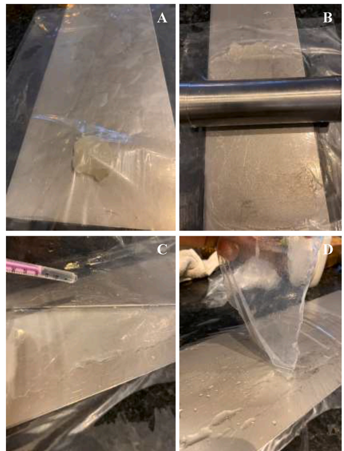
Fig. 3. Procedure for collagen film preparation. A) Collagen dispersion on a stainless-steel board between two layers of plastic sheets. B) Flattening of the collagen dispersion with a stainless-steel roller. C) Addition of saturated sodium chloride solution to the side of the collagen film, thereby gently lifting the plastic sheet. D) Collagen film precipitated with saturated sodium chloride solution.
