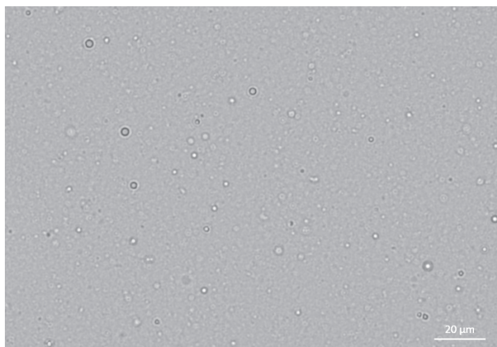
Figure S3.3 Images of Pellet obtained from 4 °C phase separation. The scale bar corresponding to 20 μm.
