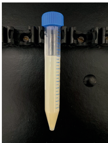
Figure S3.1 MBPSC solution ultracentrifuged at 10,000 g for 30 min.
