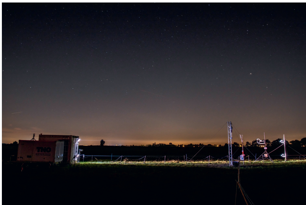
Figure 6.2: The miniDOAS NH 3 flux measurement setup at the Ruisdael Observatory at Cabauw during the RITA-2021 campaign. The light-path emitted by the miniDOAS instruments is clearly visible at night, with the miniDOAS instruments being housed in the container on the left and the retroreflectors at 22 m distance on the mast on the right. (Picture taken by Arnoud Apituley, September 2021)
