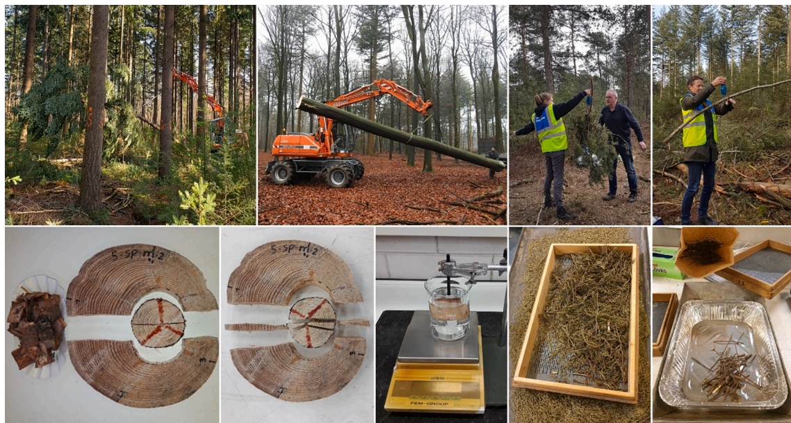
Fig. 2. Pictures of measurements in the field (top) and in the laboratory (bottom). Fieldwork included measurement of the fresh weight of the entire tree (top left), fresh weight of the stem (top middle left), fresh weight of branches (top middle right) and fresh weight of the coarse branch (top left). Laboratory work included separation of the stem disk into bark, sapwood and, if present, heartwood (bottom left), extracting slices for determination of the dry weight density (bottom middle) and separation of the dried branch material into needles (bottom middle right) and small branches (bottom right).
