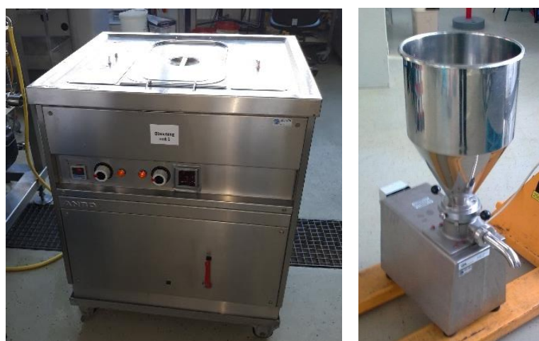
Figure 5 Blanching unit (L) and colloid mill (R) used for large scale processing of mussels
