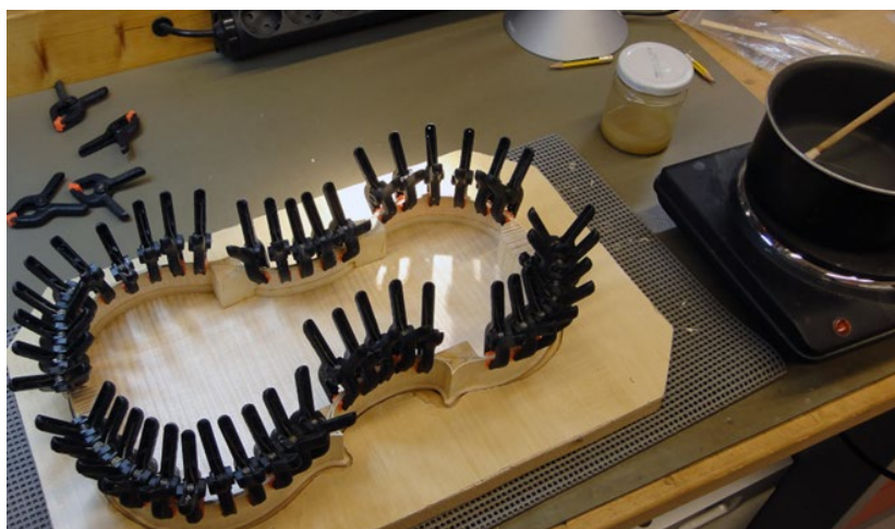
Figure 3.6. Hide glue (in the glass jar) is still the glue of choice for modern violin makers as its properties are unmatched by synthetic glues. (Photo: Arjen Bosch)
