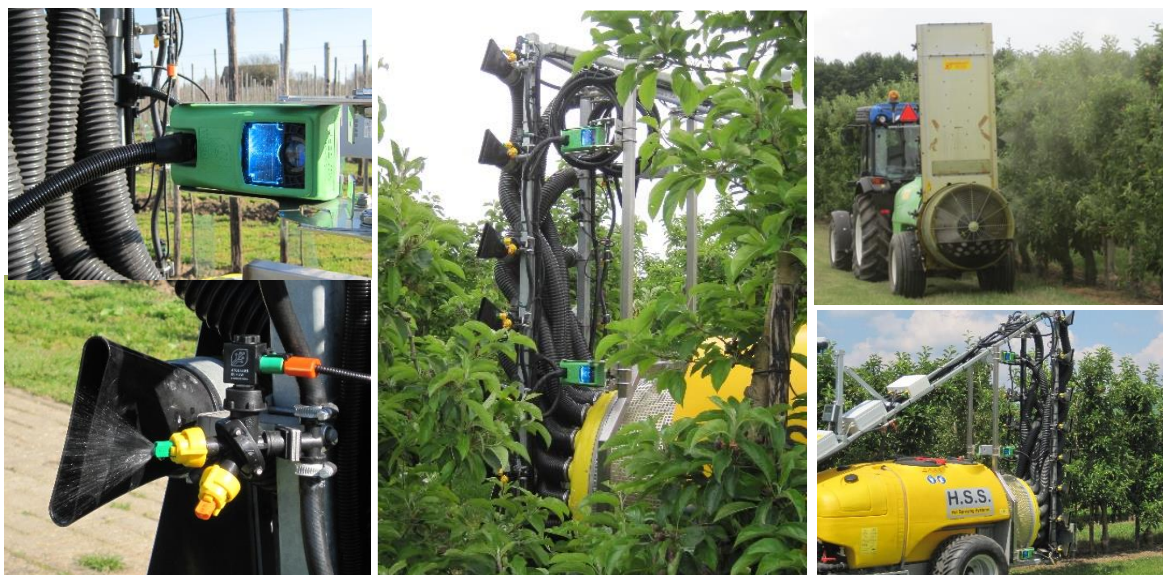
Fig. 1. Reference cross-flow fan sprayer (right top) and H.S.S.-CF I.S.A. precision sprayer (right bottom) with detail of the Rometron green detection sensor (left top) and the Rometron PWM nozzle module (left bottom) switching of nozzles if a gap between trees is detected (centre).
