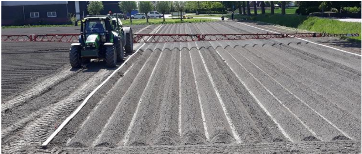
Fig. 2. Lay-out of the spray deposition collectors in the field on top of the bare potato ridges.
