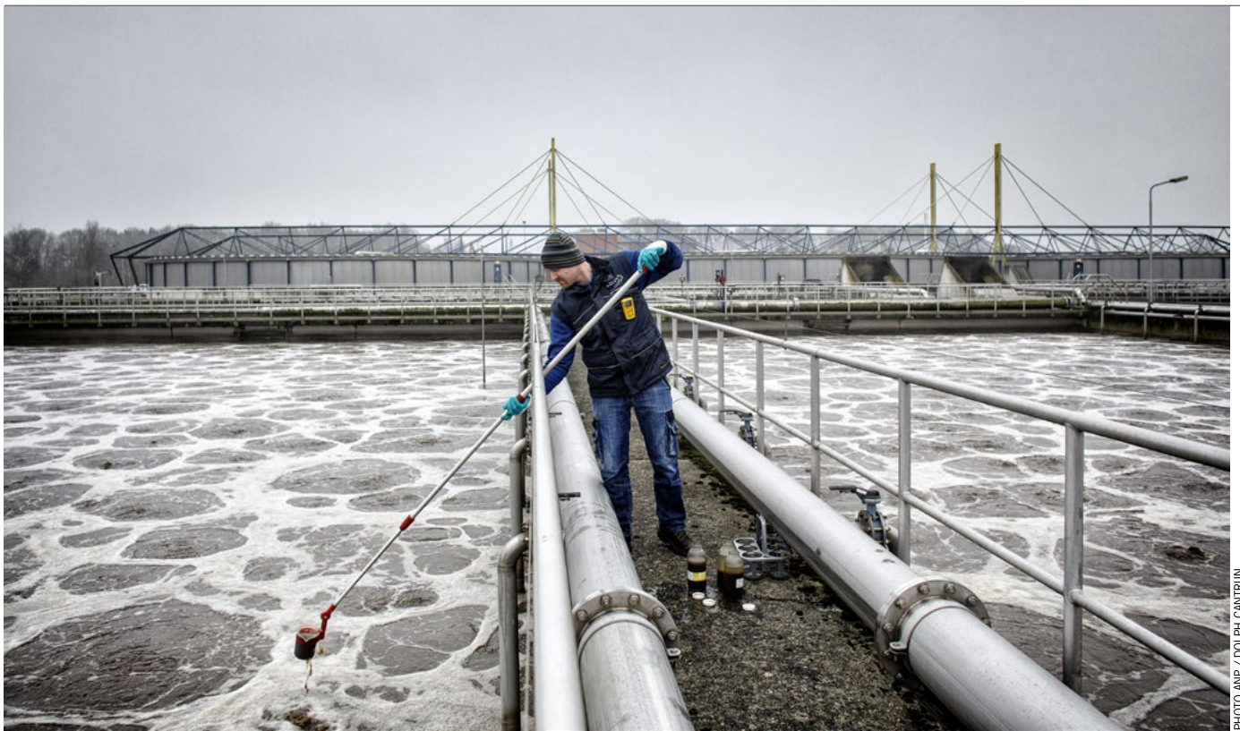
Wastewater at the sewage treatment plant in Tilburg is being tested for levels of phosphate, nitrate, ammonium and dry matter.
