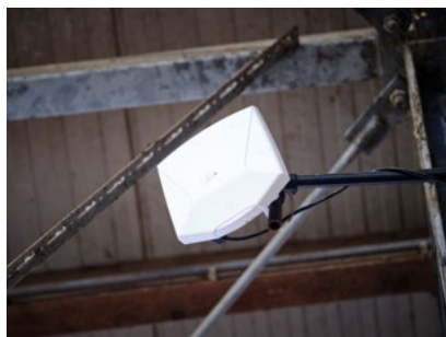
Anchors receive signals from the tags and track the position of individual cows.
