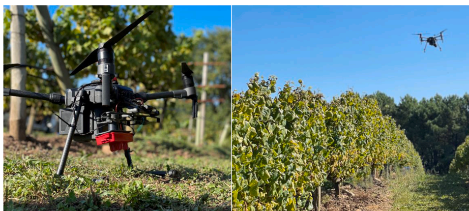
Fig. 3. Left: Unmanned Aerial System (UAS) composed of DJI M210 and Micasense RedEdge 3 multispectral camera. Right: Unmanned aerial vehicle (UAV) flight and detail of the vineyard and vegetation cover.
