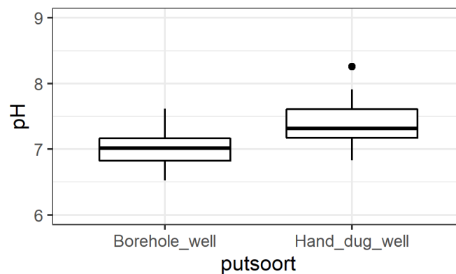
Figure A.4: Boxplot of the pH range for the borehole and hand-dug wel.
