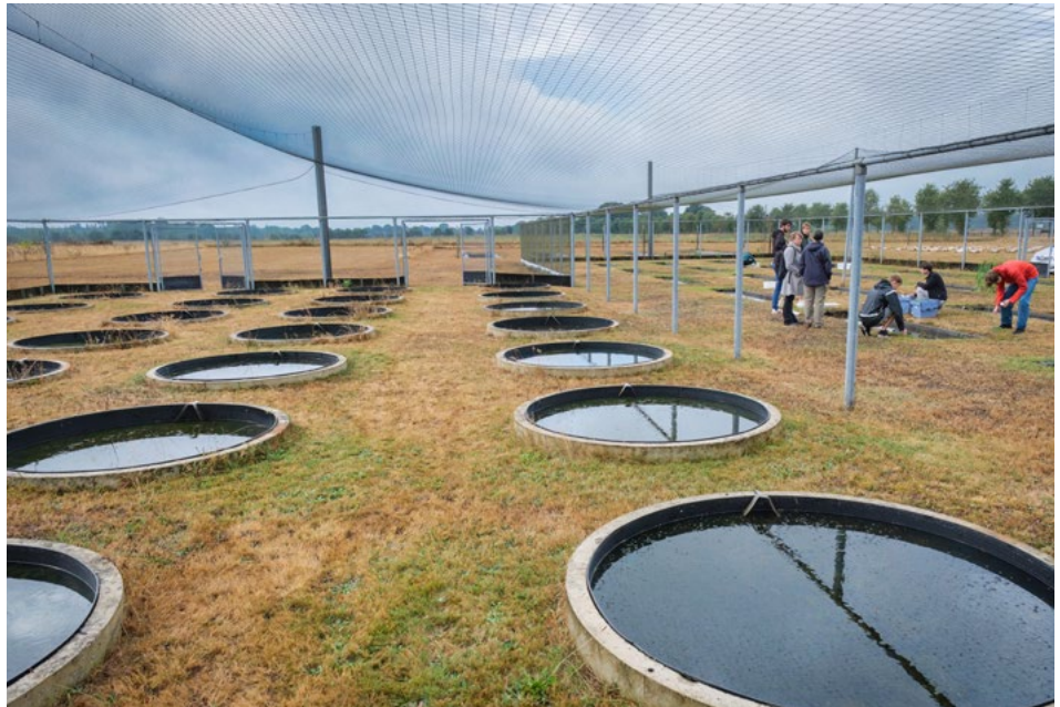
The artificially constructed test ponds and ditches at Sinderhoeve in Renkum.
