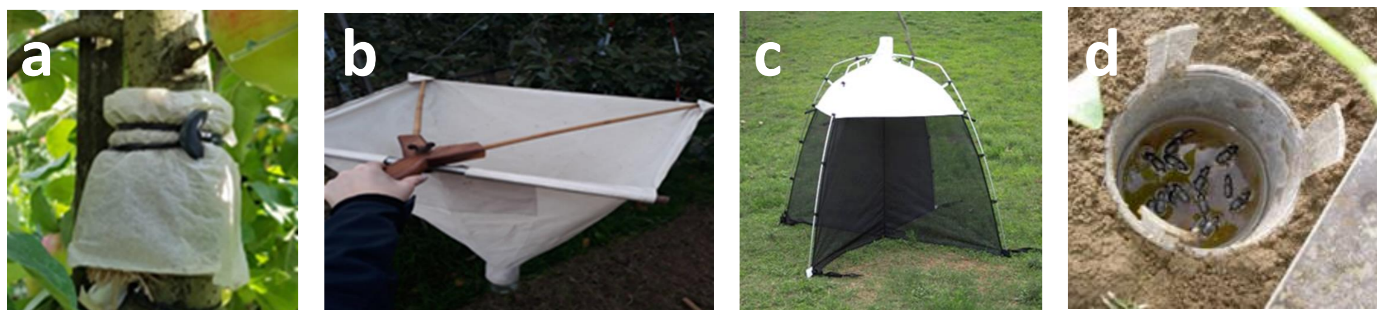
Figure 1 a-d. Different sampling techniques were used to cover arthropod subcommunities in agro-ecosystems. Limb jarring (a), beating net (b) Malaise (c) pitfall trap (d).
