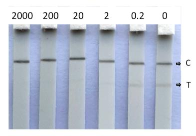
**Figure 6.** Visual detection of CHLP ( $\mu$ g/L) in fortified diluted fresh lime tree honey with C indicating the control line and T indicating the test line.
