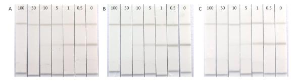
**Figure 2.** Sensitivity testing of the CHLP LFIAs by applying CHLP standards (0.5 to 100  $\mu$ g/L) in three independent runs (**A–C**) within one day with a two hour interval between each run.
