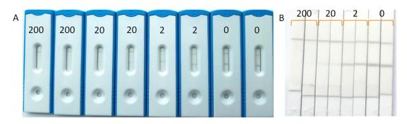
**Figure 4.** Surface water from a brook (Wageningen, The Netherlands) fortified with CHLP at 200, 20, 2, and 0  $\mu$ g/L and applied to the LFIAs in duplicate. Visual imaging was performed in the assembled cassettes (**A**) and with strips removed from the cassettes for digital imaging (**B**).
