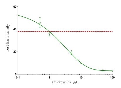
**Figure 3.** Dose–response curve constructed by four-parameter logistic regression, based on Cube readings (n = 2) of calibration standards (n = 3) in the CHLP LFIAs, performed in three independent experiments within one day with a two hour interval between each experiment, displayed as average test line intensities (n = 6). The calculated limit of detection is indicated by the red dotted line.
