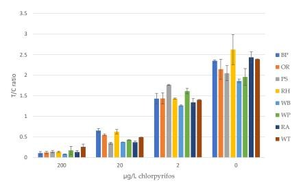
**Figure 5.** Average T/C ratios for all the CHLP fortified water samples. BP = Pond, Brussels; OR = Rhine, Oosterbeek; PS = Seine, Paris; RH = Harbor, Rotterdam; WB = Brooke, Wageningen; WP = Pond, Wageningen; AQ = aquaponics water, Rome; and T = tap water.
