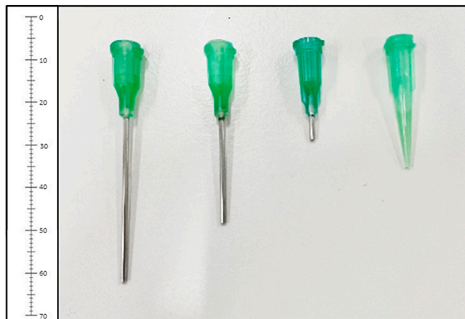
Fig. 2. Nozzle tips used for extrusion and printing. Nozzles from left to right: long straight nozzle (metal part 38.1 mm), medium straight nozzle (metal part 25.4 mm), short straight nozzle (metal part 6.35 mm) and tapered nozzle (31.2 mm). All nozzles have outlet diameter of 0.84 mm.
