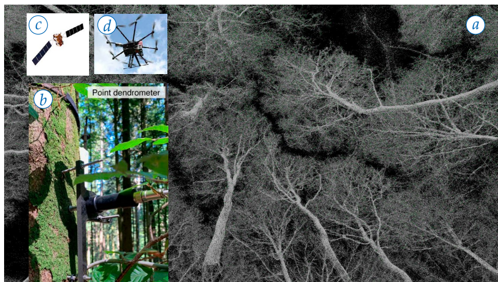
Figure 7. Examples of the equipment toolbox. a) Lidar images quantifying 3D forest structure, b) a dendrometer showing stem growth and shrinkage (proxy for water deficit) at 10 minute resolution, c) satellites and d) drones for monitoring forest dynamics from remote.
