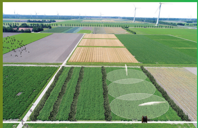
Figure 9| The irrigation of field crops with hose and reel traveling sprinkler or lateral move irrigation. The wider spacing of tree strips makes the irrigation of field crops more efficient and feasible.
