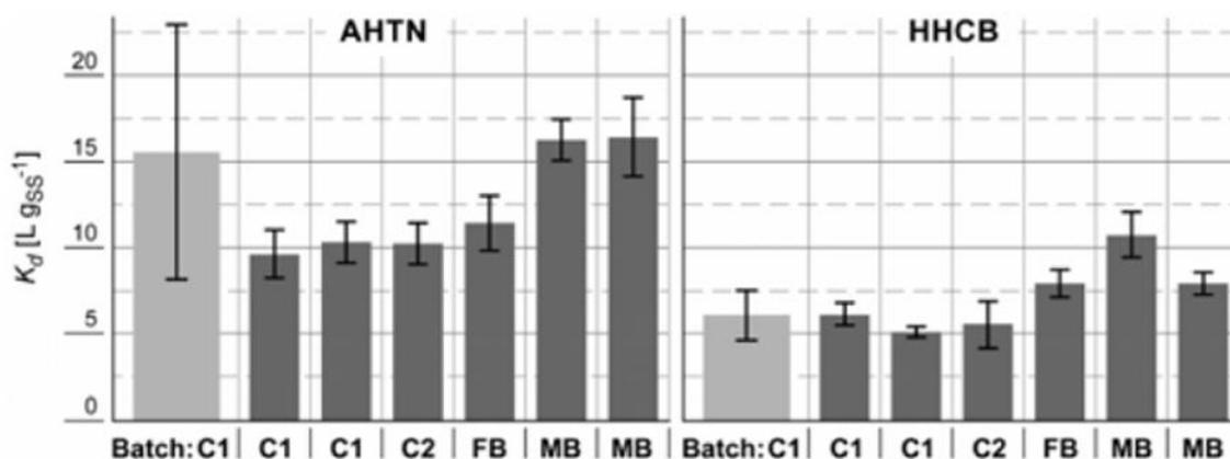
Figure 1-  $K_d$  values of musk fragrances AHTN and HHCB, obtained at different WWTPs with the following systems: C1 and C2- CAS; FB- fixed bed biofilm reactor; MB- MBR. Errors bars indicate standard deviation in 3 measured samples. Batch refers to measurements done in batch experiments, with all remaining ones being taken directly from WWTP plants. Source: Joss et al. (2006) referring to McArdell et al. (2005).
