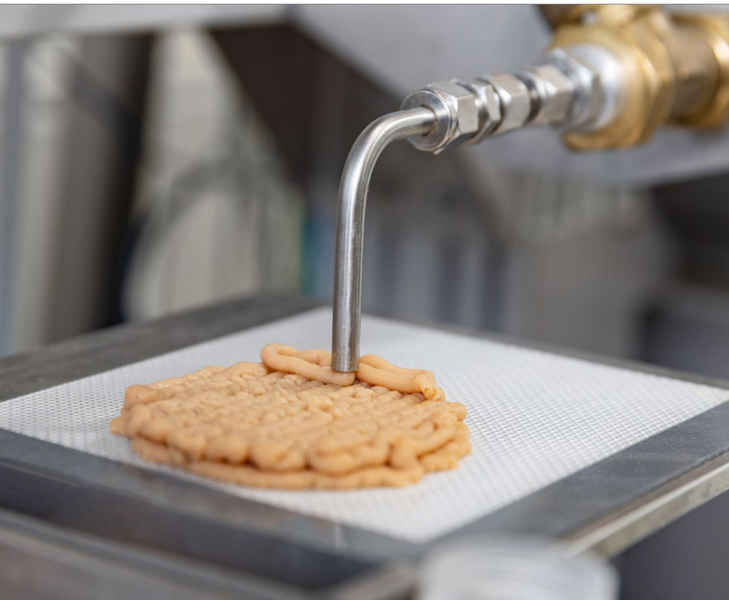
The 3D printer PSP prints a plant-based burger made up of several layers to give it a good 'bite'.
