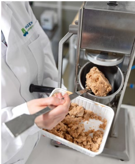
The soft dough of plant-based proteins is inserted into the printer using a 'sausage stuffer'. Processing conditions, such as the temperature, duration and cooling, can be adjusted to change such characteristics of the burger as the firmness, bite and flavour.
