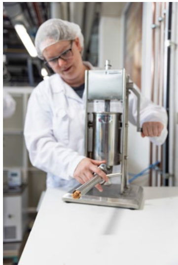
The soft dough of plant-based proteins is inserted into the printer using a 'sausage stuffer'. Processing conditions, such as the temperature, duration and cooling, can be adjusted to change such characteristics of the burger as the firmness, bite and flavour.
