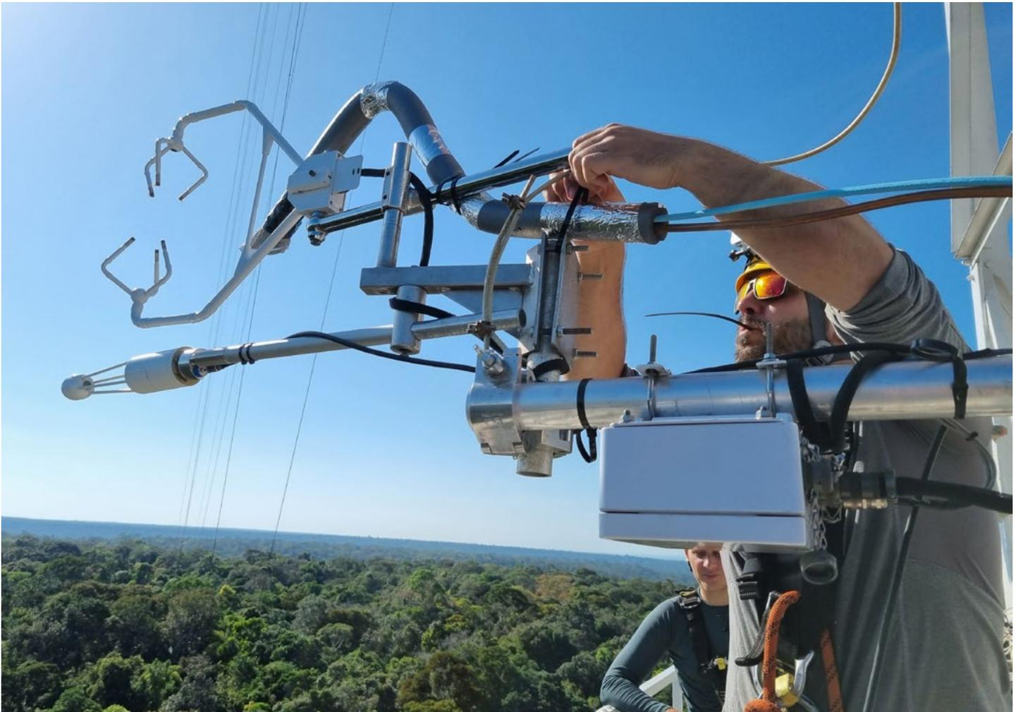
Technician David Bonell Fontas (Utrecht University) sorts out the equipment in the measurement mast. This set-up can measure the transport of CO<sub>2</sub>, H<sub>2</sub>O and their isotope composition. • Photo Oscar Hartogensis
