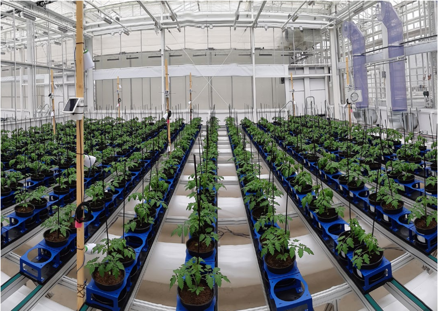
In the first section of the NPEC greenhouse on the Wageningen campus, the plants are moved on conveyor belts towards cabinets full of measuring systems. • Photo Guy Ackermans
