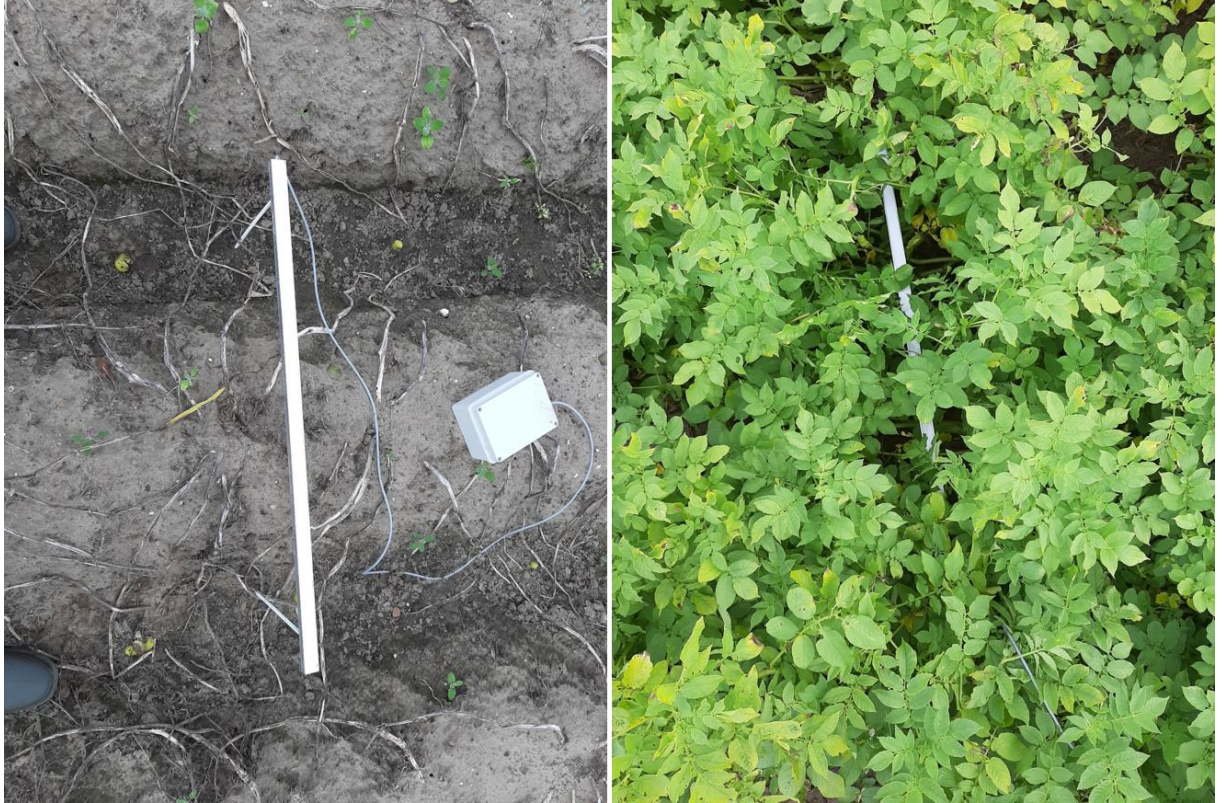
Figure 3: Sensors in the field. On the left the parbars at the end the end of the season at the bottom of the canopy and on the right in the middle of the season at the bottom of the canopy.
