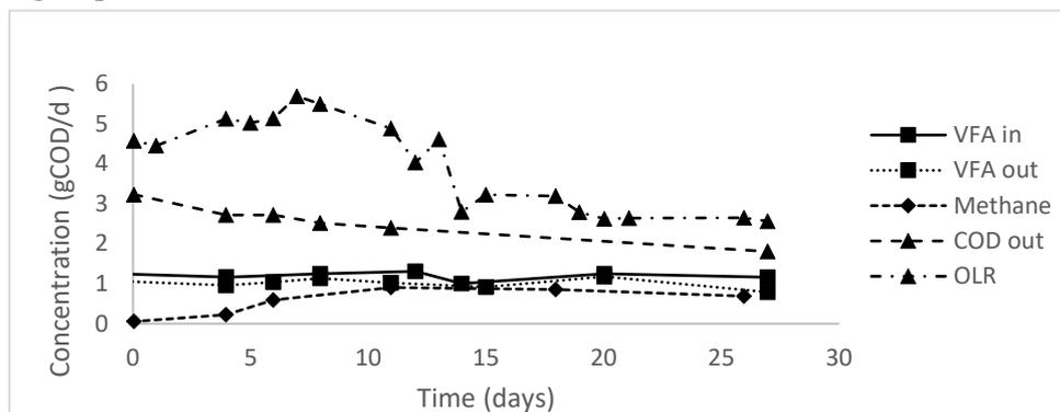
Figure 1 Influent and effluent COD total and VFA COD concentrations and methane production of the UASB reactor.
