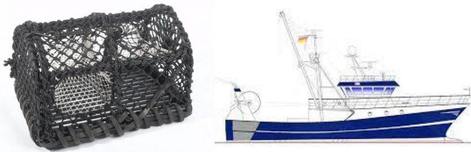
Figure 10: Crab pot (Medley) 24 inch with two side entrances as used by Dutch fishermen and stern cutter on the right.
