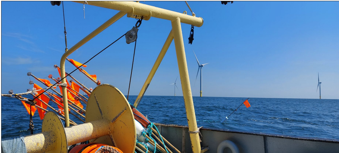
Figure 11: Deployment of a crab-pot-string in Borssele II. The dahns are the indicator of both endings of the crab-pot-string. Dahs are equipped with radar reflector and flash light (see laying dahns at the left side).
