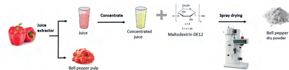
Figure 7.2 Schematic overview of the split-stream processing of red bell peppers. Red bell peppers are pressed and separated into juice (top) and bell pepper pulp (bottom). The juice is concentrated through membrane processing during which the red colour got lost. The concentrated juice is mixed with maltodextrin DE12. This mixture is dried into a fine bell pepper powder using the Büchi B-290 spray dryer.
