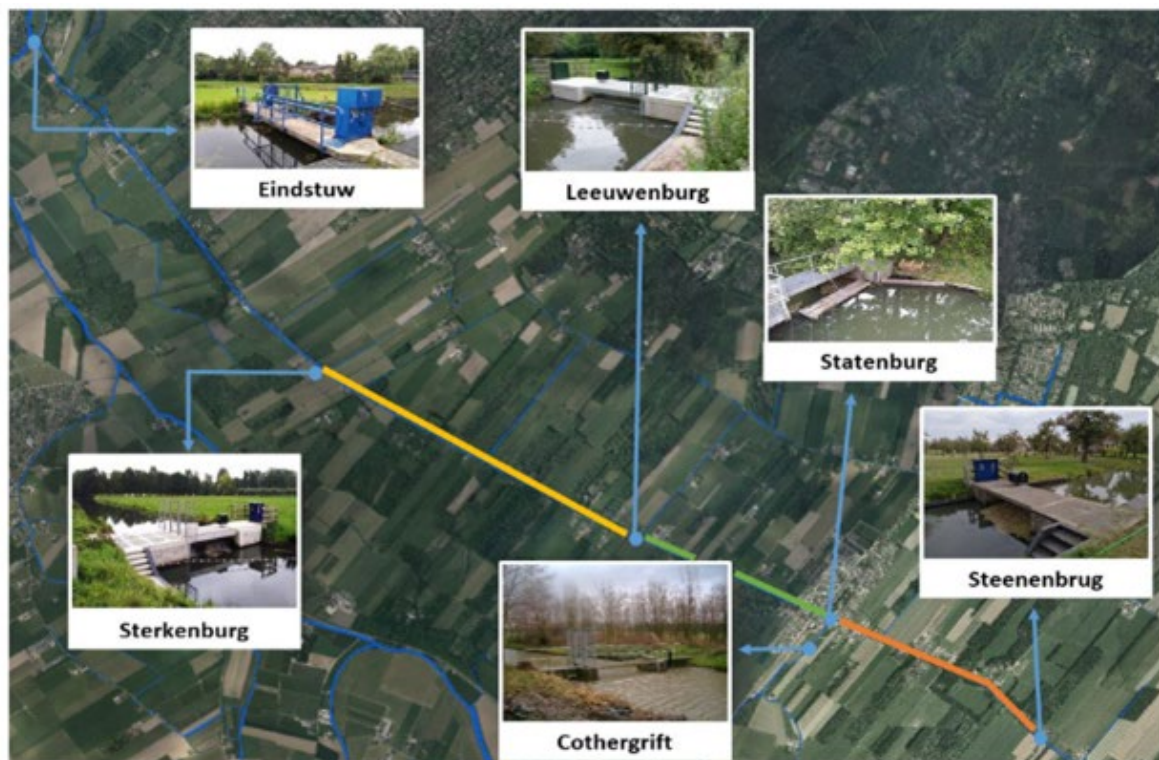
Figure 3.3. Overview of the weirs in the Langbroekerwetering where detection stations were installed. Including the division of four compartments: blue: A:Eindstuw-Sterkenburg, yellow: B:Sterkenburg-Leeuwenburg, green: C:Leeuwenburg-Statenburg and orange: D:Statenburg-Steenenbrug-Cothergrift.
