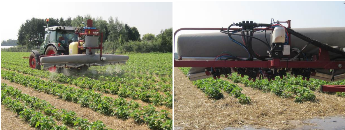
Fig. 1. CDS sprayer in strawberry (left) with adapted air sleeve and nozzle orientation to focus on strawberry plant rows on top of each bed (right).
