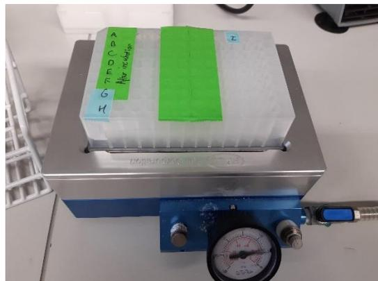
Figure S3. Some cells are taped off to increase suction.
