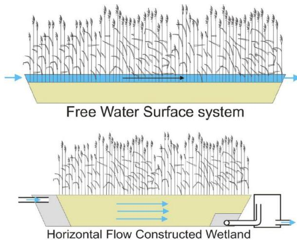
**Figure 1** Side-view of a) Surface flow (upper) and b) Sub-surface horizontal flow (lower) wetland
