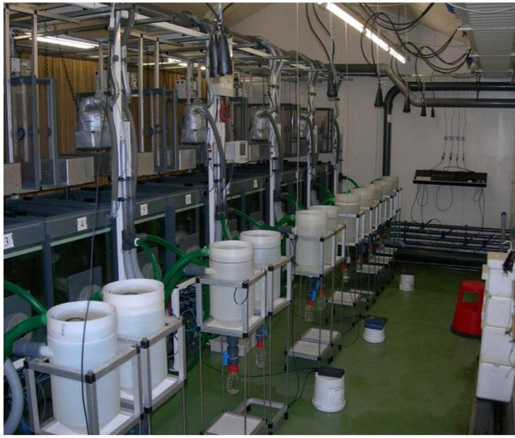
**Figure 1. Research facility to determine faecal loss of fish** (Photo: Aquaculture Research Facility, CARUS, Wageningen University)
